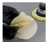
enables the removal of the Rhynogrip discs from the machine's backing pad for reuse.
